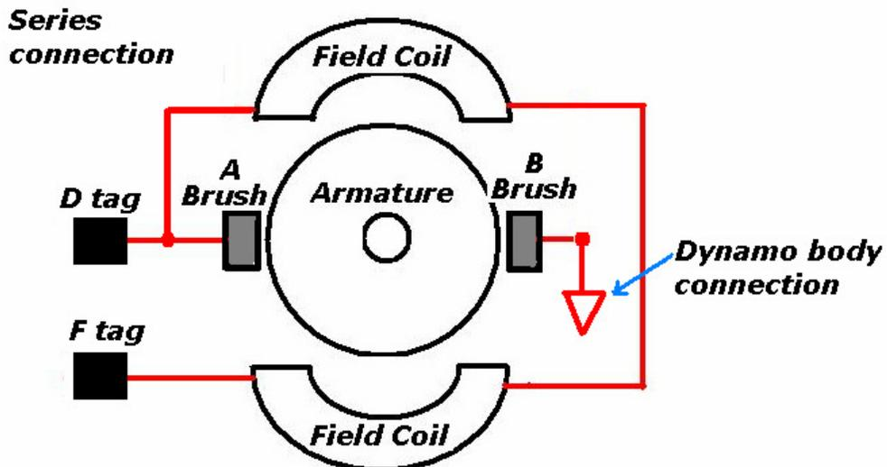
wire and work out if there are just one connection to a brush (in which case it's most likely a series connection) or if there are 2 wires in which case it's most likely a shunt connection.
